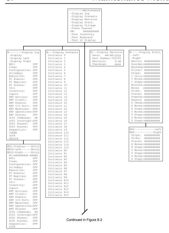
Figure 8-1 The TLS Maintenance Menu (Part 1)
